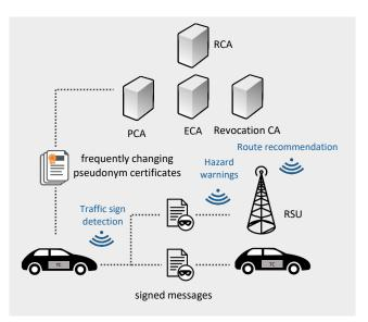
Figure 1: A V2X security solution based on PKI
