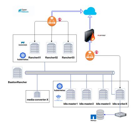
Figure 3.1: CSUC Deployment Scenario
