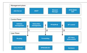
Figure 3.8: BNG Control and User Plane Separation
