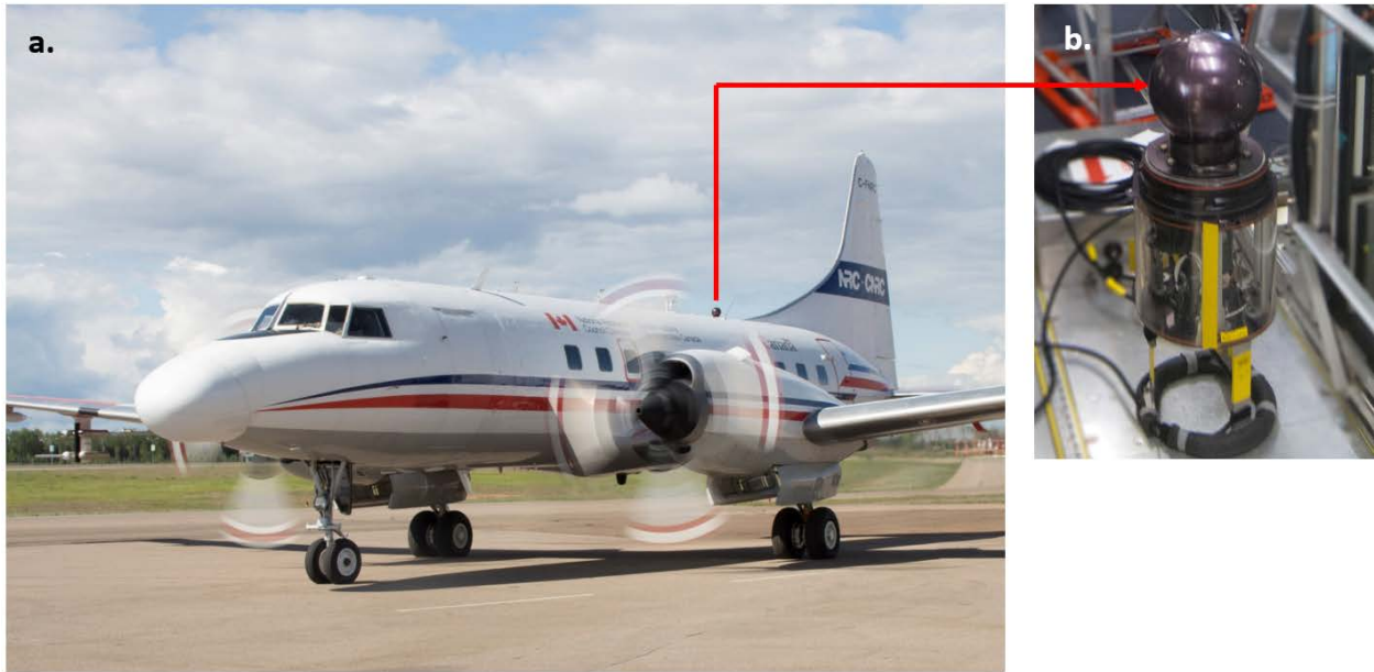
Figure 3. a. 4STAR at Fort McMurray installed on the Convair-580 aircraft; b. 4STAR head and its optical cables sitting inside the aircraft
