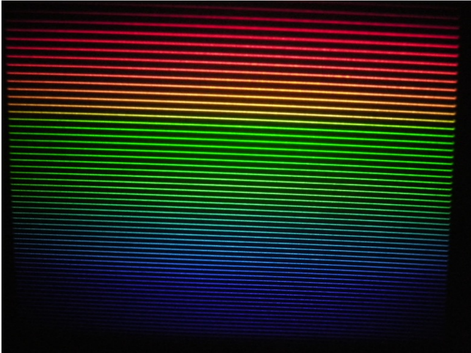
Figure 4: (Pre-) first light spectrum obtained by HARPS-N. The horizontal bands are the wavelength orders split by a grating, each of which is then split by a grism. This setup produces thousands of spectral lines, from which a precise RV measurement can be extracted. Picture captured by Francesco Pepe with a DSLR camera.
