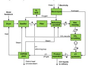
**Figure 3:** FLEXCHX process with electrolysis boosting and FT off-gas recycling.
