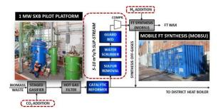
**Figure 4:** Pilot-scale experimental facilities used for validating the key enabling technologies.
