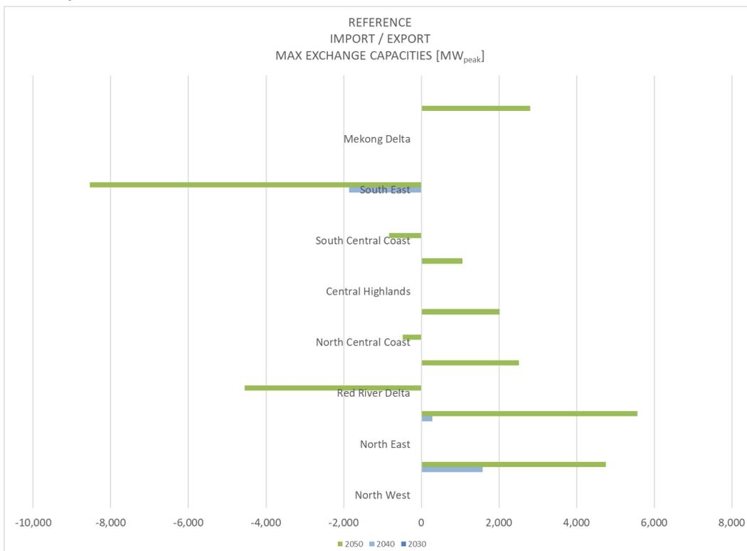
**Figure 32: Viet Nam: Maximum interregional exchange capacities—additional to the required grid capacity expansion in response to load increase—under the RENEWABLES 1 scenario**
