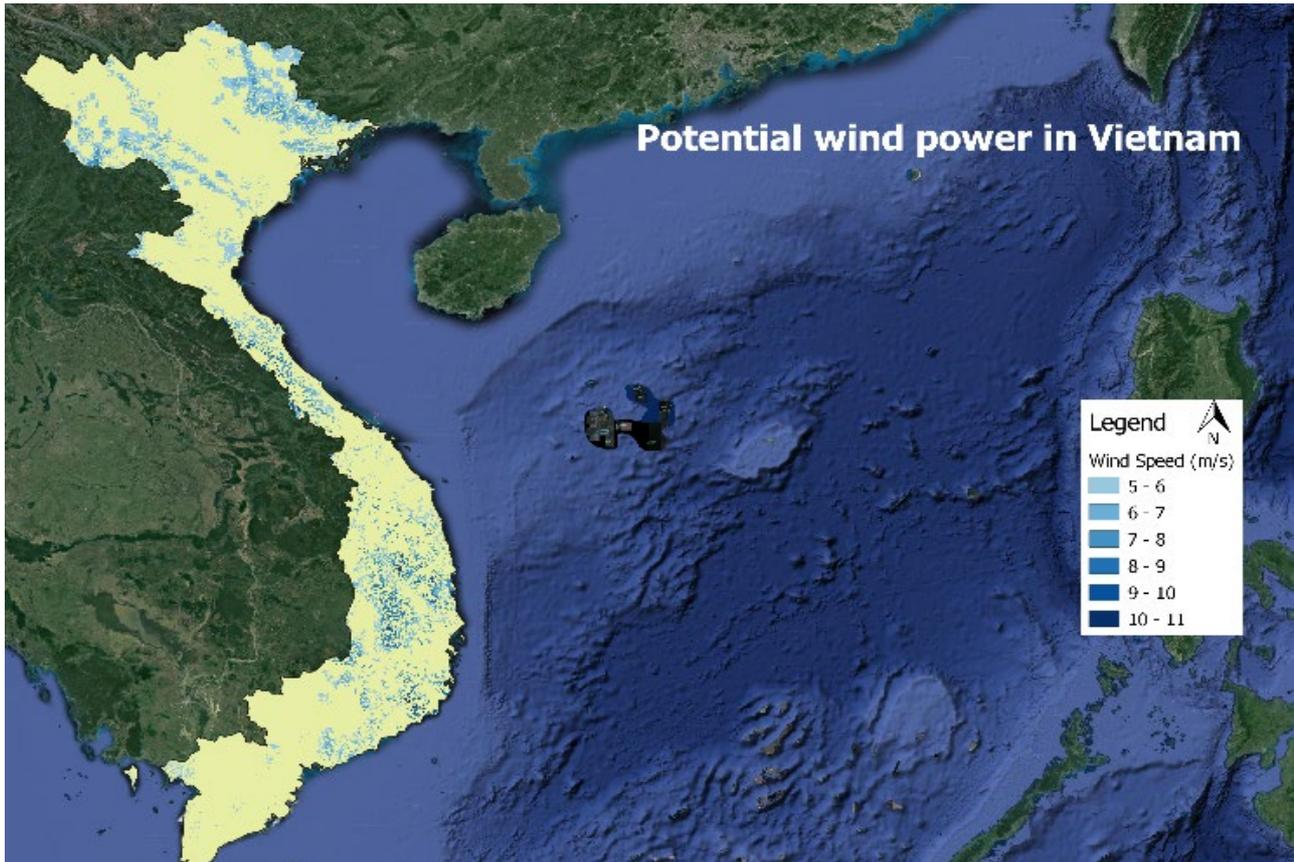
Figure 14: On- and offshore wind energy generation potential in Viet Nam
