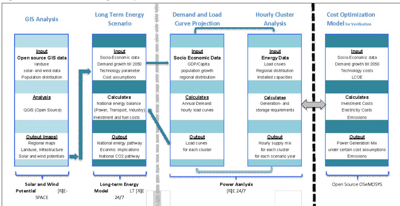
In the mapping analysis, a global information system (GIS) was used for the regional analysis of Viet Nam’s population density and distribution, its solar and wind resources and the currently existing energy infrastructure (transmission power lines and power plants with over 100 MW installed capacity). This information has been used to define the cluster breakdown.
