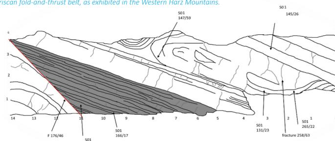
Fig.5 – digitised field sketch of classic Variscan thrust and NW verging fold interaction. Possibly internal folding.
