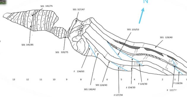
Fig.4 – image (right) and digitised field sketch (above) of Variscan fold and thrust interactions, no visible hinge but hinge can be implied. High level of deformation in the overturned limb.
