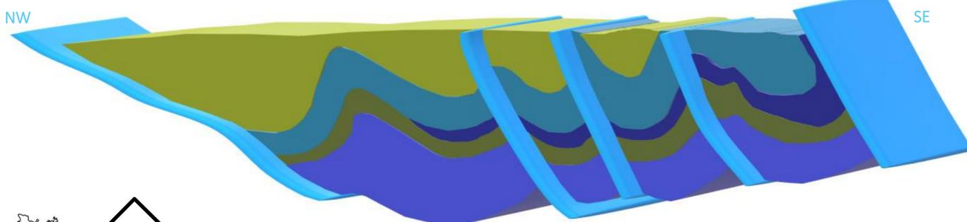
Fig.2 – Simplified conceptual 3D diagram of Variscan fold-and-thrust belt, as exhibited in the Western Harz Mountains.
