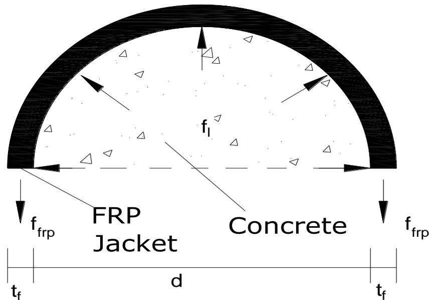
*Figure 1: Free-body diagram of FRP jacket.*
