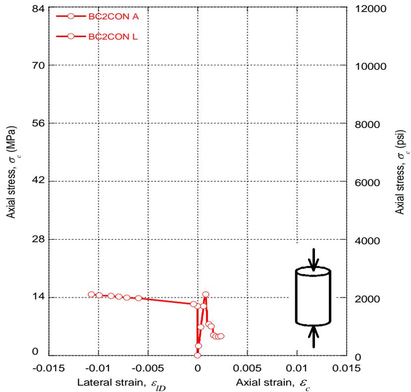
**Figure 7:** Evaluation of axial stress v/s axial strain and axial stress v/s lateral strain behavior of unconfined circular plain brick concrete column of size 2.
