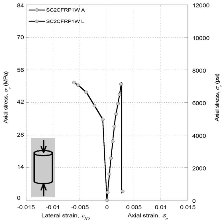
**Figure 12:** Evaluation of axial stress v/s axial strain and axial stress v/s lateral strain behavior of CFRP confined plain stone concrete column of size 2.
