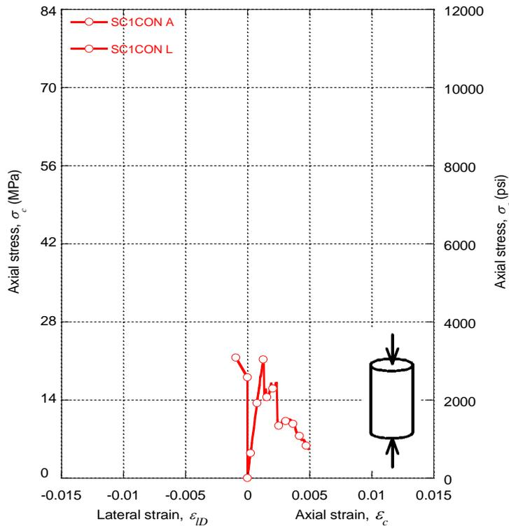
**Figure 9:** Evaluation of axial stress v/s axial strain and axial stress v/s lateral strain behavior of unconfined circular plain stone concrete column of size 1.
