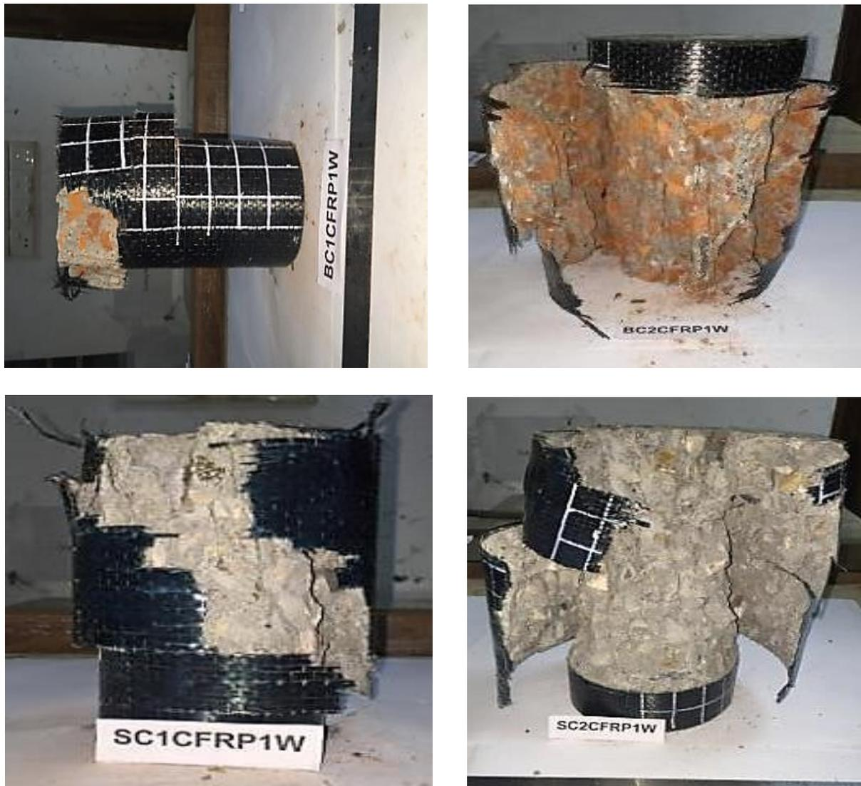
*Figure 13: Failure pattern of (a) BC1CFRP1W, (b) BC2CFRP1W, (c) SC1CFRP1W and (d) SC2CFRP1W sample.*
