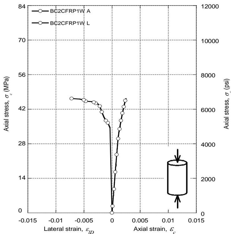
**Figure 8:** Evaluation of axial stress v/s axial strain and axial stress v/s lateral strain behavior of CFRP confined plain brick concrete column of size 2.
