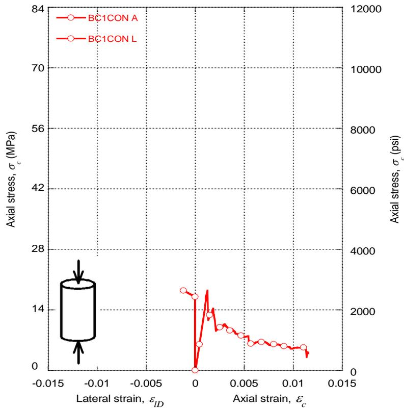
**Figure 5:** Evaluation of axial stress v/s axial strain and axial stress v/s lateral strain behavior of unconfined circular plain brick concrete column of size 1.
