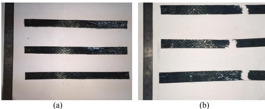
**Figure 4:** CFRP tensile test specimen (a) before and (b) after the test.
