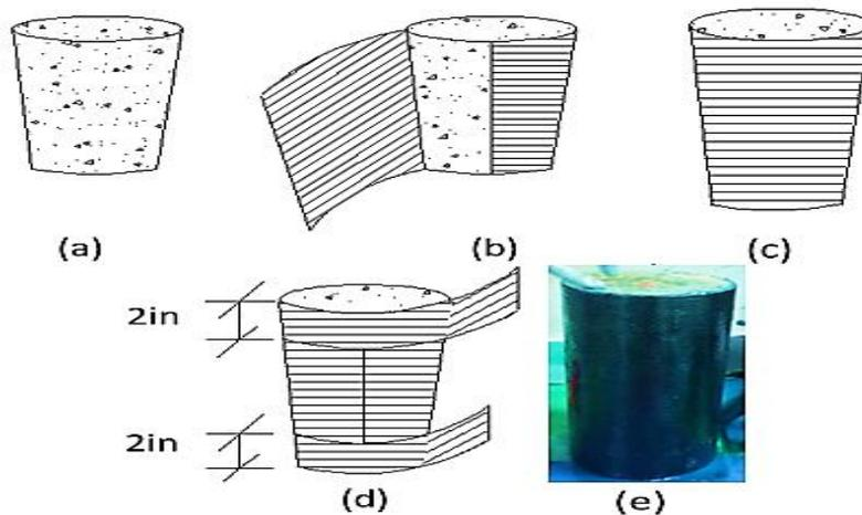
**Figure 2:** (a), (b), (c), (d) Schematic diagram of the wrapping process of CFRP on size 2 specimen and (e) One layer of CFRP wrapped column.
