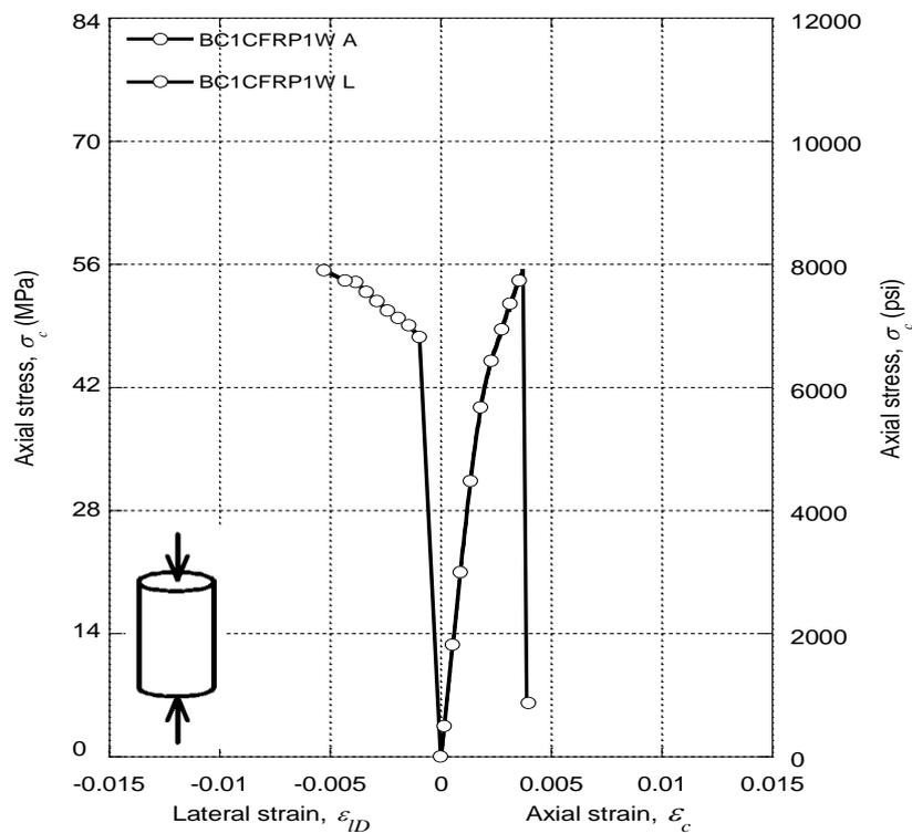
**Figure 6:** Evaluation of axial stress v/s axial strain and axial stress v/s lateral strain behavior of CFRP confined plain brick concrete column of size 1.
