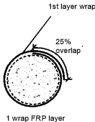
**Figure 3:** Typical layout of FRP wrapped specimen.
