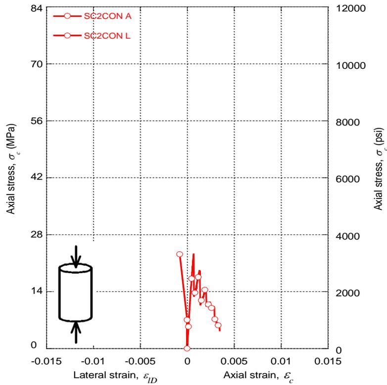
**Figure 11:** Evaluation of axial stress v/s axial strain and axial stress v/s lateral strain behavior of unconfined circular plain stone concrete column of size 2.
