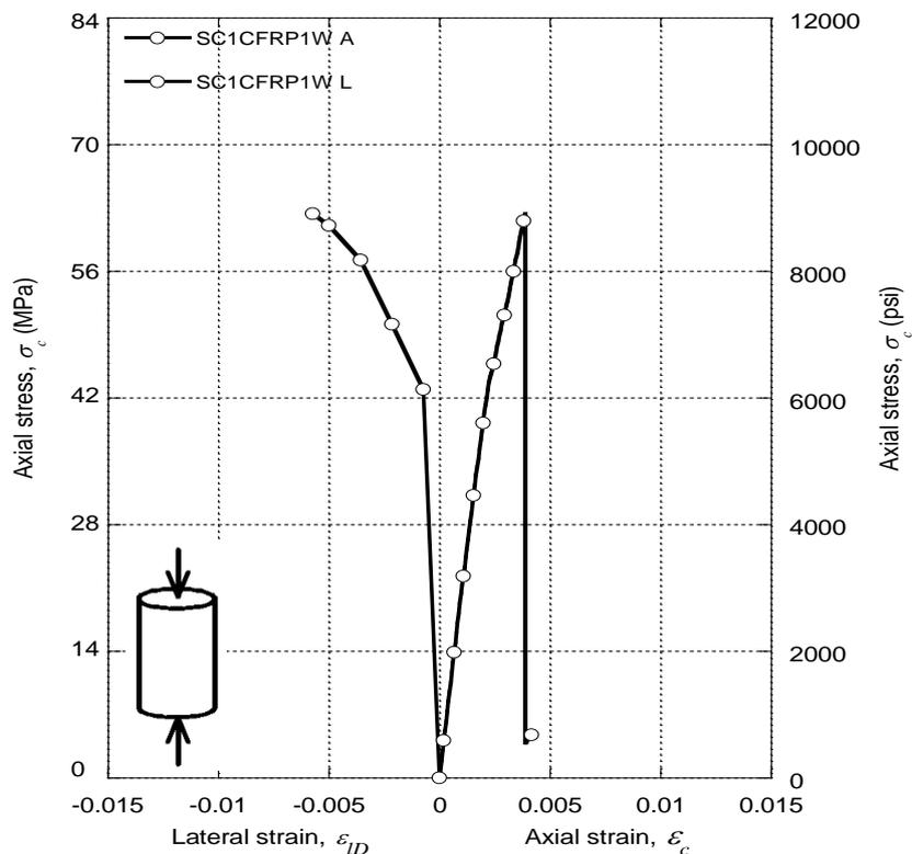
**Figure 10:** Evaluation of axial stress v/s axial strain and axial stress v/s lateral strain behavior of CFRP confined plain stone concrete column of size 1.
