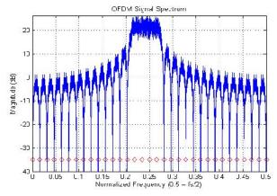
Fig8. OFDM signal spectrum
