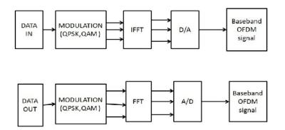
Fig2. OFDM Transmitter and receiver block diagram.
