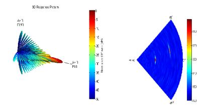
Fig13.rectangular array pattern
