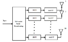
Fig3. Beam forming in OFDM radar transmitter block
