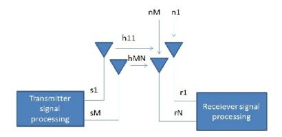
Fig1. M-Transmitter and N-Receiver Multiple antenna configuration.
