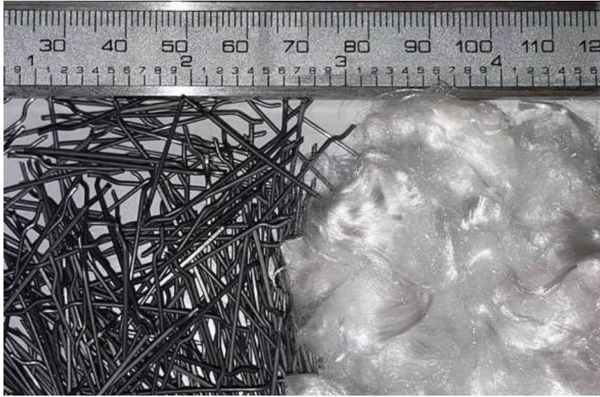
Figure 1: Hooked-end steel macrofibers and polypropylene microfibers.
