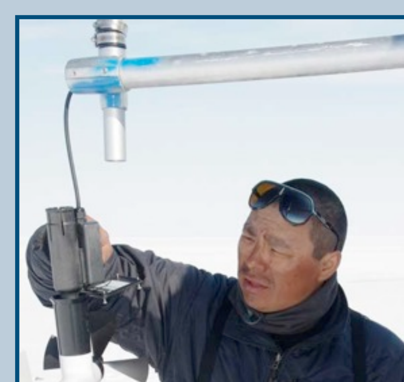
Clyde River-based researcher Esa Qillaq changes an anemometer at the northern station. Photo credit: Henry Huntington
