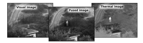
Fig. 3. Image fusion of visual and thermal images
