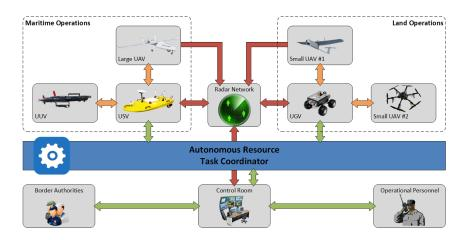
Fig. 5. Higher-level depiction of the system's architecture.
