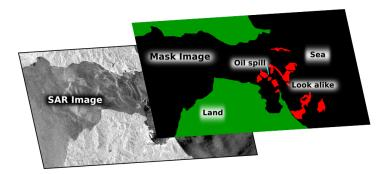
Fig. 1. SAR Image and the corresponding mask for semantic representation of the scenery
