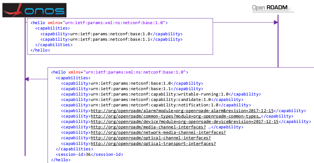
Figure 18. Initial Capability Discovery between the SDN controller and the OpenROADM
