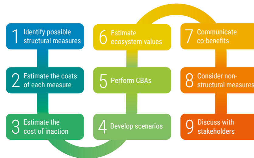
Figure 15.5 Steps identifying for green, grey/green or grey scenarios. Inspired by Rao et al. 2013. Design: K. Sudmeier
