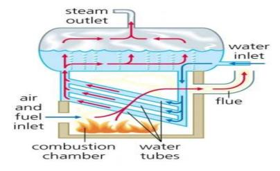
Figure 2: Process of steam production
