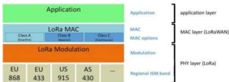
Fig. 2: LoRa vs. LoRaWAN
