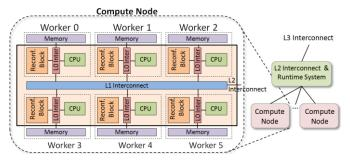
Figure 3. The ECOSCALE Hardware Architecture.
