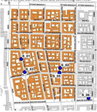
Despite general satisfying results, the noise monitoring network suffers from vandalism (one point was decommissioned) and high temperature in summer (damages to batteries of smartphones).
