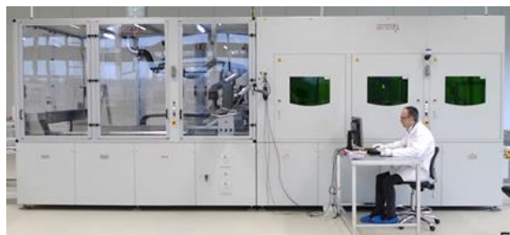
Figure 3: Multi-functional automated module layup and interconnection tool
