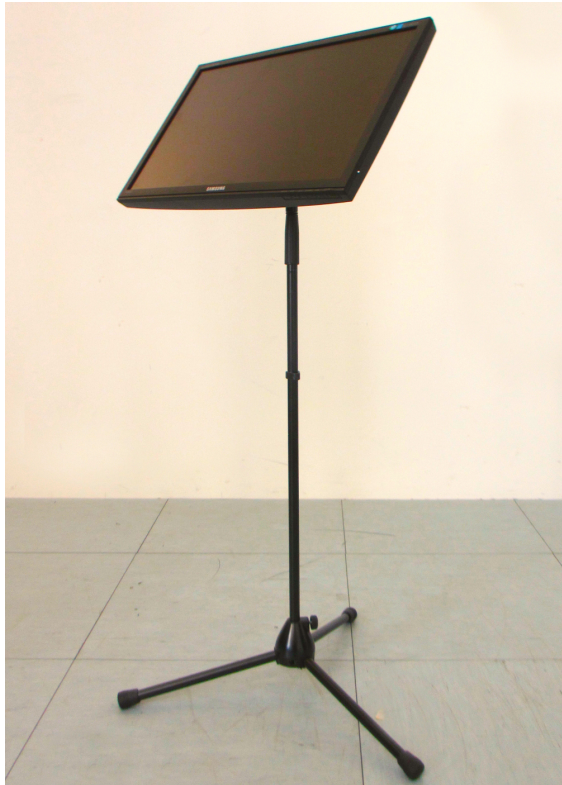
Figure 1. An electronic music stand consisting of a 24” screen mounted on a microphone stand.
