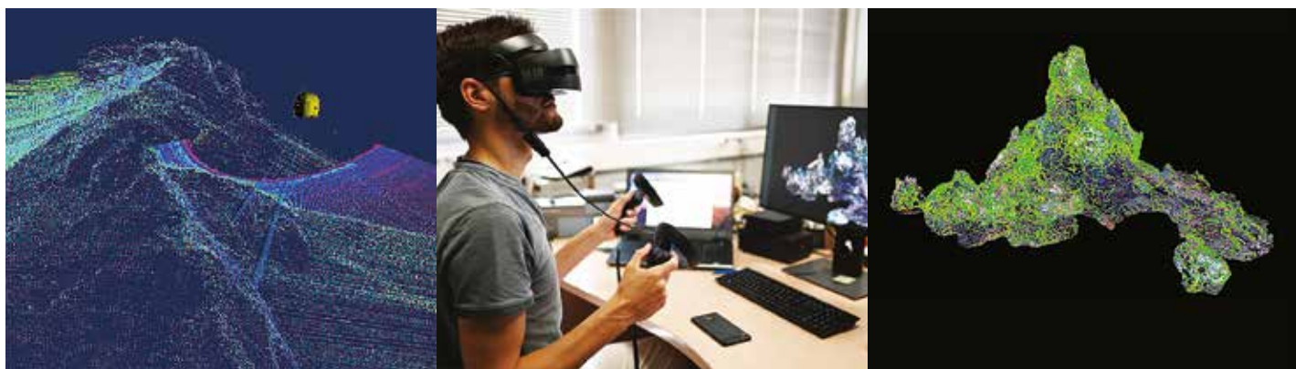
Left: real time 3D modeling from multibeam echosounder data and visualization of the vehicle (here HROV Ariane ) with respect to the seabed; Centre: 3D immersive viewing and analyzing of optical terrain model; Right: classification during scientific post-processing the same 3D terrain model
