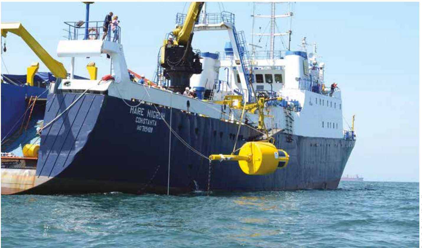
RV Mare Nigrum deploying an in situ observing buoy
