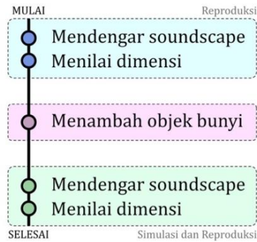
Gambar IV.7 Alur prosedur uji dengar soundscape di laboratorium.
