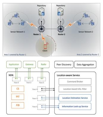
Figure 1. The proposed design and the major components of NDN-based Location-aware architecture
