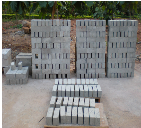
Figure-1: a. atmospheric curing of geopolymer fly ash building brick (at 35°C)
