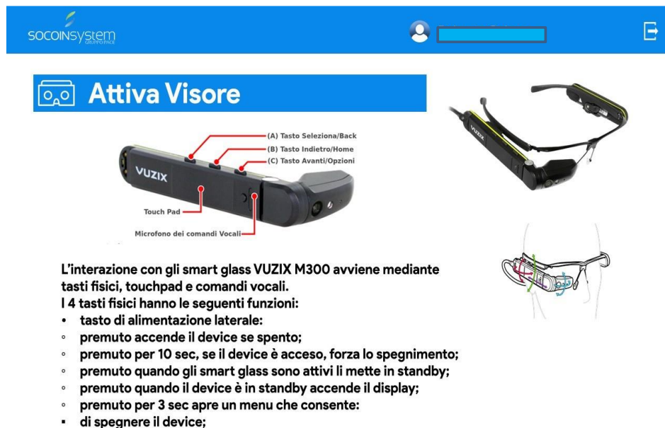
Figure 7. Example of procedures to configure the Vuzix smart glasses.
