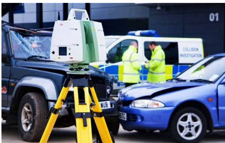
Figure 4: 3D Laser scanner crowd points of Accident Scene
