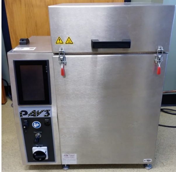
Figure 2. Pressure aging vessel (PAV).
