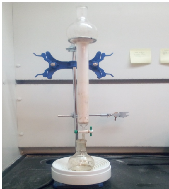
Figure 13. Separation of aromatics, resins, and asphaltenes.
