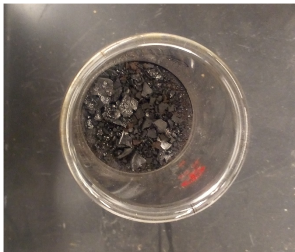
Figure 12. Separation of asphaltene.
