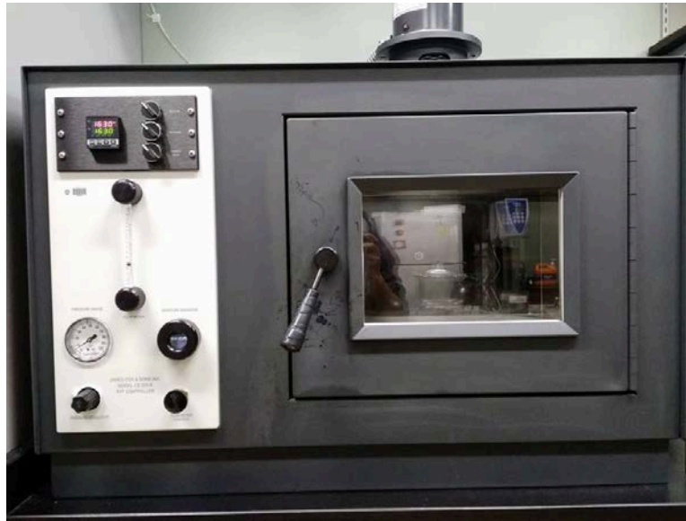
Figure 1. Rolling thin film oven.
