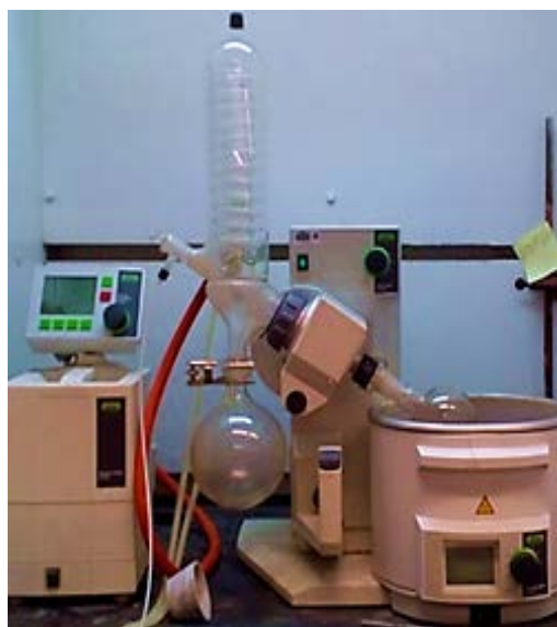
Figure 14. Evaporation of solvent with a rotary evaporator.
