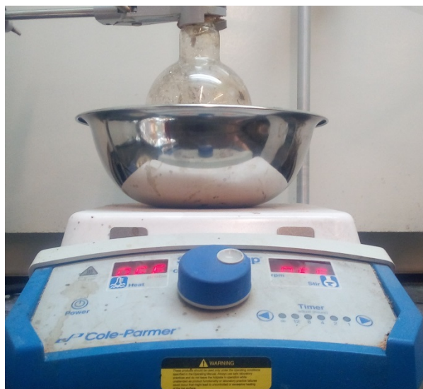
Figure 11. Dissolving asphalt on n-heptane.
