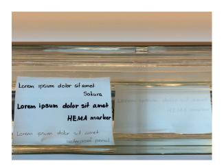
Output from test at Picturae with iPhone. By using only 1 pixel, the back of the label also comes out legibly, in mirror image.
