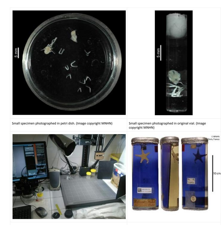
Imaging station for sealed containers: monitor with live view and camera left, specimen and background right. Black paper is used to limit lighting to relevant parts. (Image copyright MNHN)
