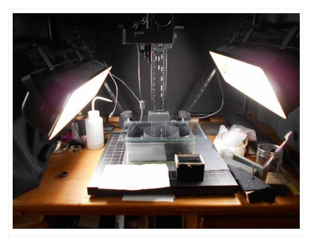
Photography setup for dry imaging of liquid preserved specimens: the specimen is placed on the glass pane, which is raised from the background, to ensure a blurred background. The camera is facing down on a copy stand and two lights are on either side. (Image copyright MNHN)
