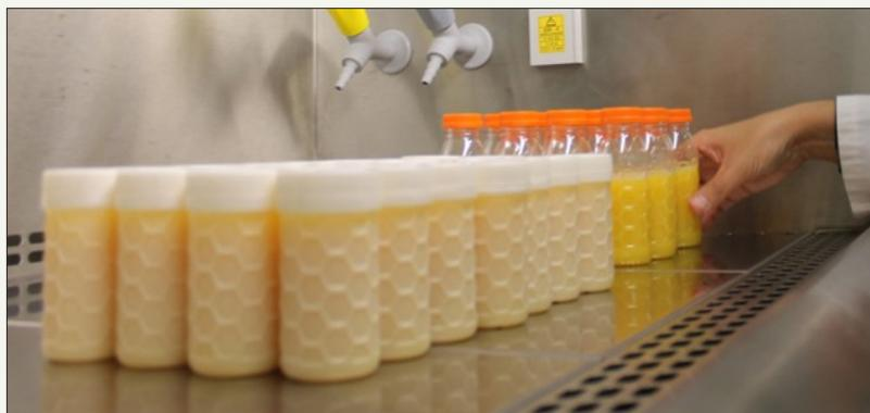
**Figure 2:** Bottles made from PHA [23].
