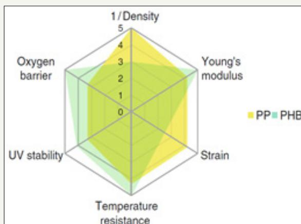
Figure 1: Diagram comparing PHB and PP reproduced [7].
