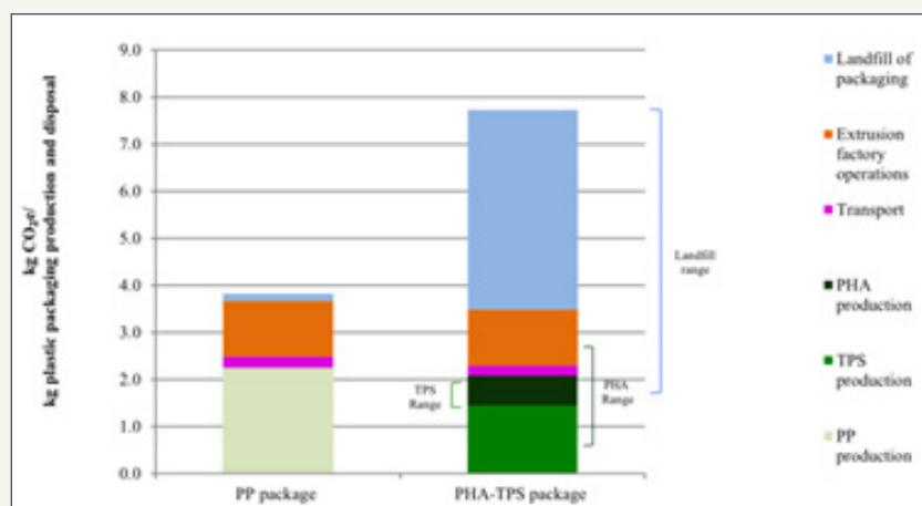
**Figure 4:** Kg CO<sub>2e</sub> emissions (GWP100) for the production and disposal of 1kg of PP or PHA-TPS food packaging. GWP100=greenhouse warming potential with a 100-year horizon.
