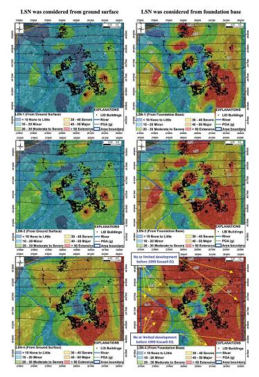
Figure 5. Comparison of LID buildings and Liquefaction Severity Number (LSN) maps for Adapazari considered from ground surface and foundation base conclusions
