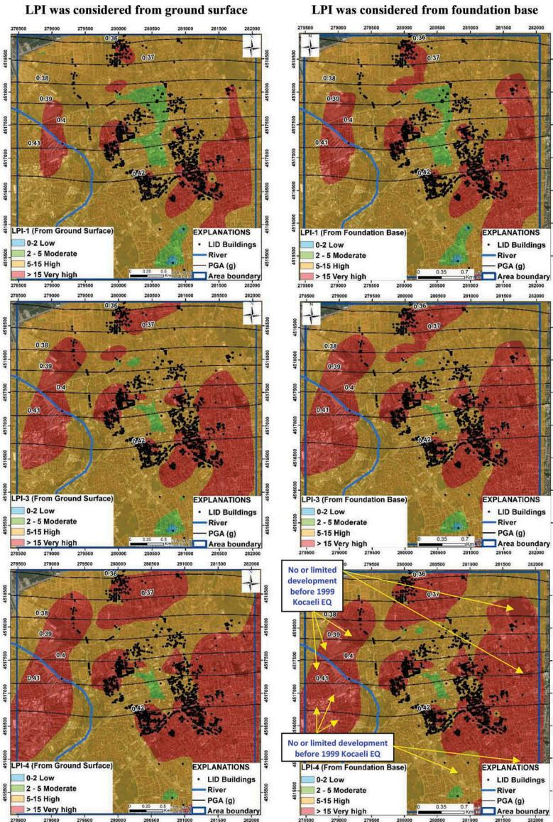
Figure 4. Comparison of LID buildings and Liquefaction Potential Index (LPI) maps for Adapazari considered from ground surface and foundation base
