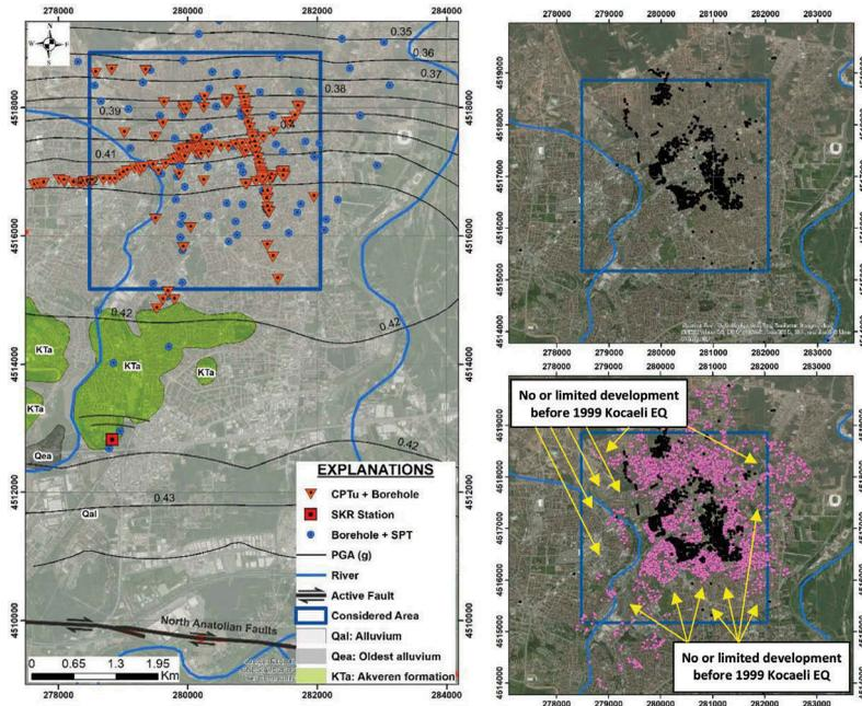
Figure 2. (a) Geology and seismic demand map including field investigations, (b) Liquefaction Induced Damage (LID) buildings, (c) All damaged buildings in Adapazari following the 1999 Kocaeli Earthquake
