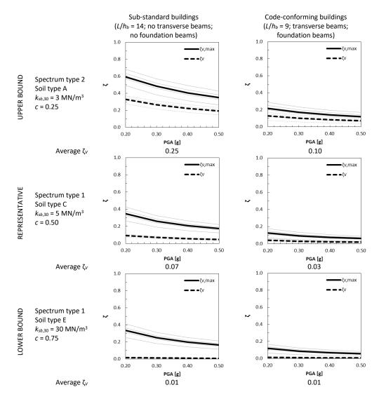
Figure 9. Values of relative shear force ( $\zeta_V$ ) due to settlement depending on the PGA of the seismic event for different situations; h = 3 m,  $h_b/b_w = 1.5$ ,  $w = 6.6 \text{ kN/m}^2$ ,  $q = 100 \text{ kN/m}^2$ ; thick line denotes average values
