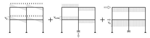
Figure 2. Maximum |V| in beams considering superposition of gravitational loading  $(V_g)$ , maximum free differential settlement of interior footing  $(V_{s,max})$  and seismic action  $(V_d)$
