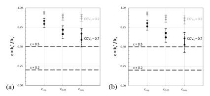
Figure 7. Representative ( $c_{rep}$ ), characteristic ( $c_{0.05}$ ) and minimum ( $c_{min}$ ) equivalent soil degradation parameter according to different geometric and probabilistic assumptions, for  $\Delta H = 4B$  (a) or 6B (b)
