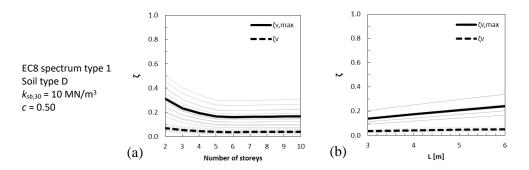
Figure 8. Values of relative shear force depending on n (a) and L (b) for sub-standard buildings
