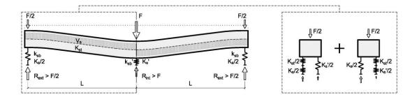
Figure 3. Conceptual model adopted for the calculation of the structure-to-soil stiffness weighting factor  $\chi$  (a) and decomposition of the static problem of each half (b)
