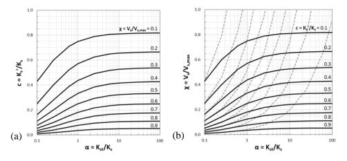
Figure 4. Charts of  $\chi$  depending on c and  $\alpha$ ; the dashed grey line shows qualitatively the greater increase of resistance (capacity) with respect to the increase of demand when the stiffness is increased
