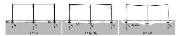
Figure 1. Conceptual configurations of equivalent models and  $\Delta S$  for decreasing values of c
