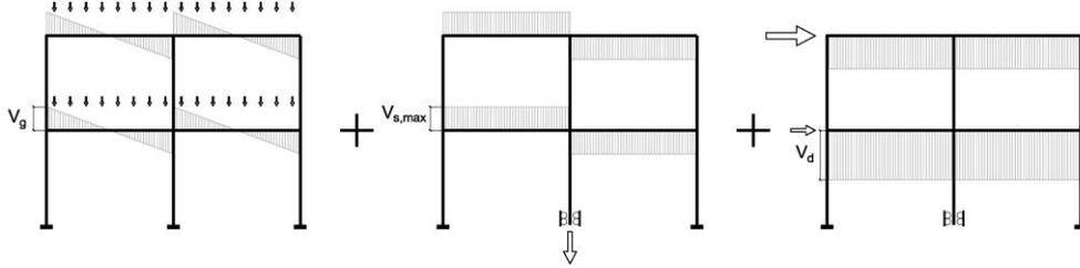
Figure 2. Maximum  $|V|$  in beams considering superposition of gravitational loading ( $V_g$ ), maximum free differential settlement of interior footing ( $V_{s,max}$ ) and seismic action ( $V_d$ )
