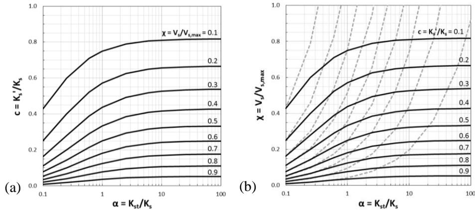
Figure 4. Charts of  $\chi$  depending on  $c$  and  $\alpha$ ; the dashed grey line shows qualitatively the greater increase of resistance (capacity) with respect to the increase of demand when the stiffness is increased
