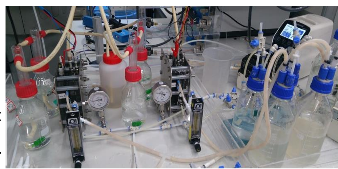
Figure 3: BES setup for nitrogen recovery
