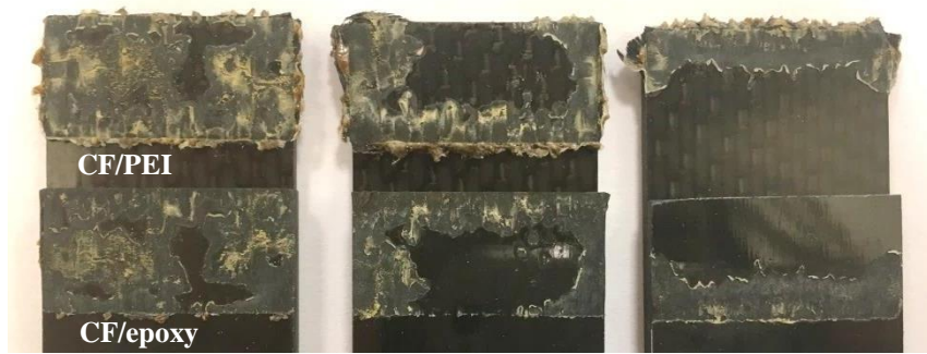
Fig 7. Fracture surfaces obtained for the ED-less welding case with the same welding parameters.
