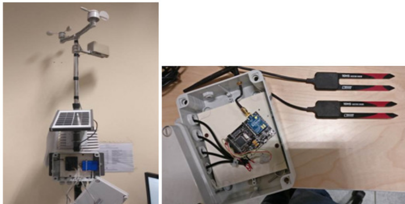
Figure 3. (Left) Final prototype System; (Right) Location of the Wasp mote Coordinator.
