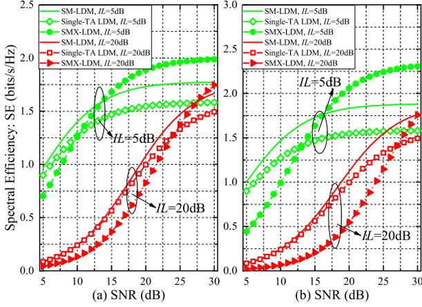
Fig. 5. The SE performance of FL in SM-LDM, single-TA LDM and SMX-LDM systems versus SNR with  $N_{\text{m}} = 2$ ,  $N_{\text{r}} = 2$  and  $IL \in \{5 \text{ dB}, 20 \text{ dB}\}$ .  $N_t = 2$  in (a) and  $N_t = 4$  in (b).
