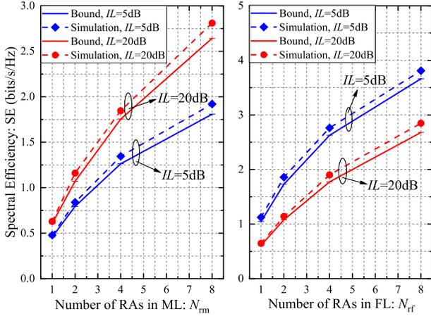
Fig. 2. The SE performance of simulation results and our proposed SE lower bound versus  $N_{fm}$  for ML in (a). The SE performance of simulation results and our proposed SE lower bound versus  $N_{rf}$  for FL in (b).
