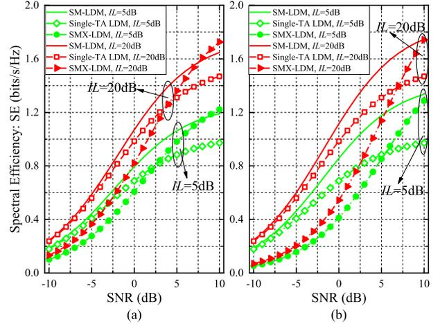
Fig. 4. The SE performance of ML in SM-LDM, single-TA LDM and SMX-LDM systems versus SNR with  $N_{fm} = 2$ ,  $N_{rf} = 2$  and  $IL \in \{5\text{ dB}, 20\text{ dB}\}$ .  $N_t = 2$  in (a) and  $N_t = 4$  in (b).
