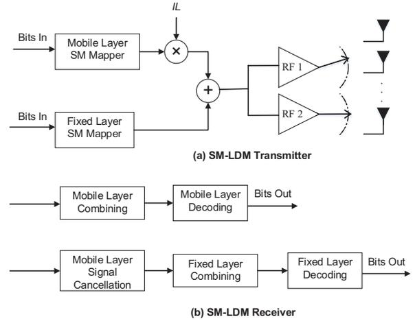
Fig. 1. Transmitter and receiver for the two-layer SM-LDM system.
