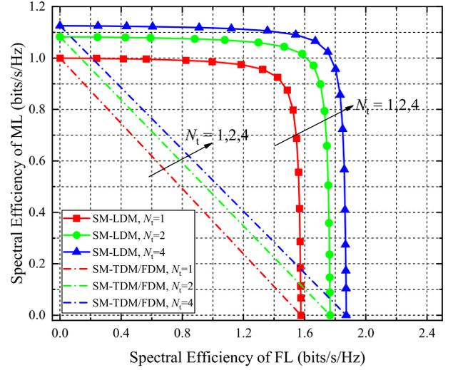
Fig. 6. The SE performance of ML and FL in SM-LDM and SM-TDM/FDM systems with  $N_t \in \{1, 2, 4\}$ ,  $N_{\text{m}} = 2$ ,  $N_{\text{r}} = 2$ ,  $\text{SNR}_{\text{ml}} = 0 \text{ dB}$  and  $\text{SNR}_{\text{fl}} = 20 \text{ dB}$ .
