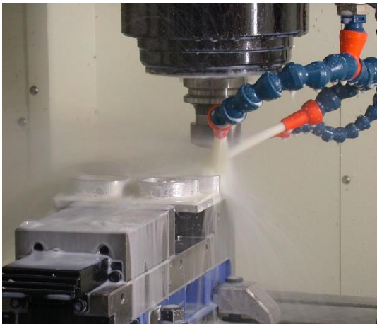
Figures 11 and 12: left: Thin-wall milling of aluminium with cutting fluid (Courtesy of Glenn McKechnie), right: Traditional vacuum-filter system for MWF (Courtesy of Eriez Hydroflow)
