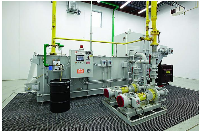
Figures 11 and 12: left: Thin-wall milling of aluminium with cutting fluid (Courtesy of Glenn McKechnie), right: Traditional vacuum-filter system for MWF (Courtesy of Eriez Hydroflow)
