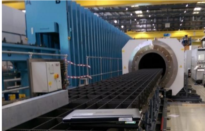
Figure 7: Furnace for thermal treatment of magnets (Courtesy of Friedrich Lackner/CERN)
