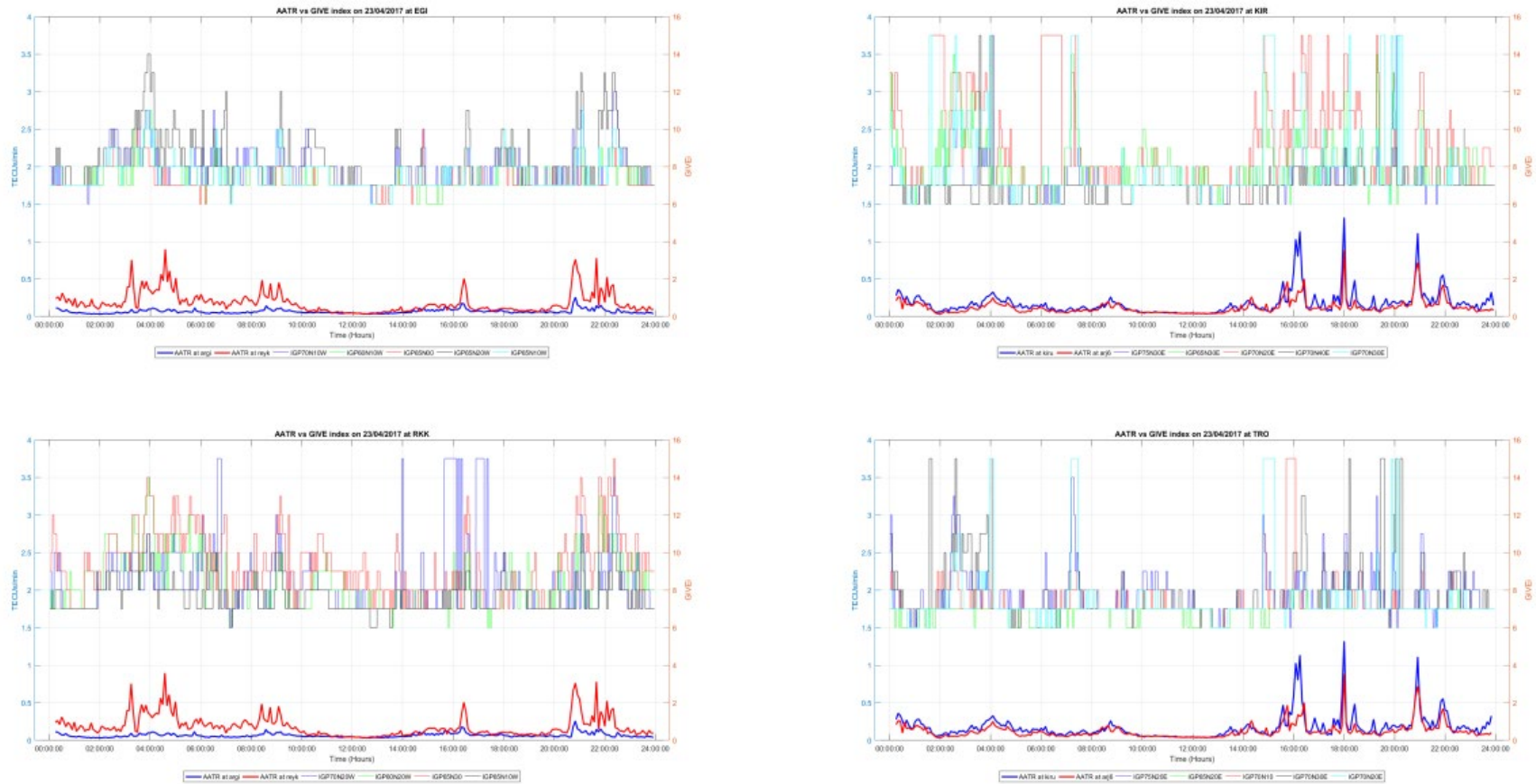
Figure 90. Temporal evolution of GIVE indices at IGPs surrounding assessed RIMS and AATR at IGS stations on DOY 113.
