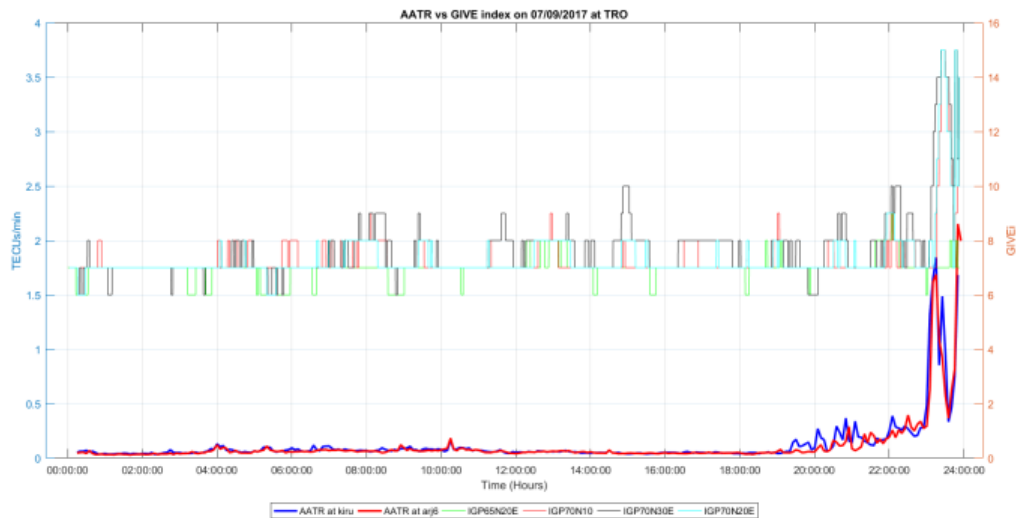
Figure 20 AATR at KIRU (in bottom blue) and ARJ6 (in bottom red) and the GIVE indices around RIMS TRO (top of the graph) on 7th September 2017.
