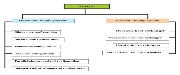
Figure 8. Common types of ground-loop heat exchangers
