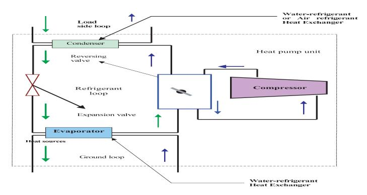
Figure 9. Schematic of GSHP system (heating mode operation)
