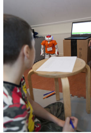
Fig. 2. Set-up of the experiment. The NAO verbally presents example scenarios and provides two explanations for each of these. The screen textually shows what the NAO is saying, so the child can always read-back what happened on the screen. The child then puts a mark at the most preferred explanation.
