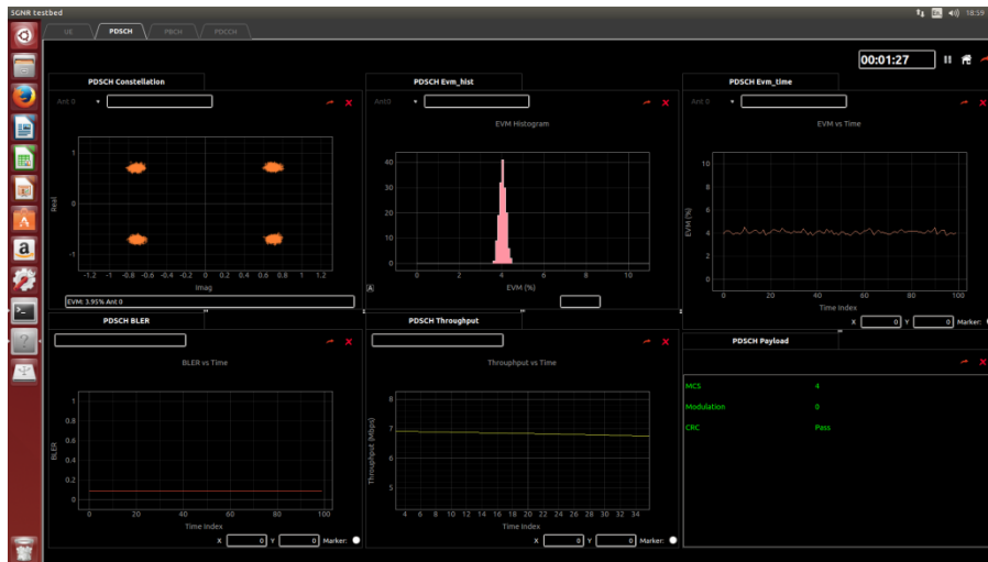
Figure C-4 Throughput of VLC with QPSK
