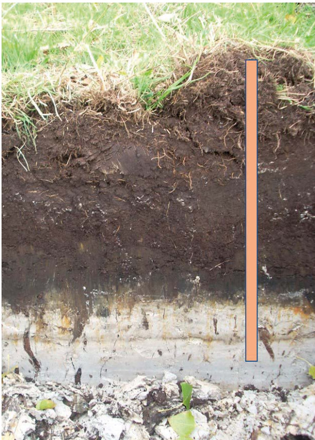
Figure 2. Assebroekse Meersen. The natural profile shows a horizon of about 45 cm thick consisting of amorphous peaty material, underlain by marl sediments with former root galleries (bar = 80 cm).
