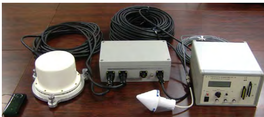
Figure 2. Current MAGDAS magnetometer system, called MAGDAS-9. This system consists of a data logging/transfer unit (right), a GPS antenna, a magnetometer main unit, a magnetic sensor, and a cellphone for reference (left), respectively. Total weight of items shown in this figure is 15.5kg. The type of geomagnetic sensor is that of 3-axial components ring-core fluxgate. It has a \pm 70,000\text{nT}/32\text{bits} dynamic range, and a 0.01\text{nT} resolution. For more details, see our website, http://www.serc.kyushu-u.ac.jp/magdas/MAGDAS_Project.htm .
