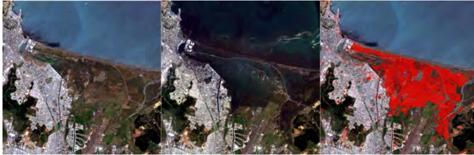
Figure 1. Damages by tsunami: City of Concepcion, Chile imaged on 10/01/2010 (left images) and 27/02/2010 (centre/right images) by the RapidEye satellite constellation. The centre image was taken eight hours after an earthquake of magnitude 8.8 had occurred and the resulting tsunami had affected the shoreline. The right map shows the areas with tsunami-related changes (red layer) on the post-tsunami image. Images courtesy of RapidEye AG, Copyright 2011, all rights reserved.
