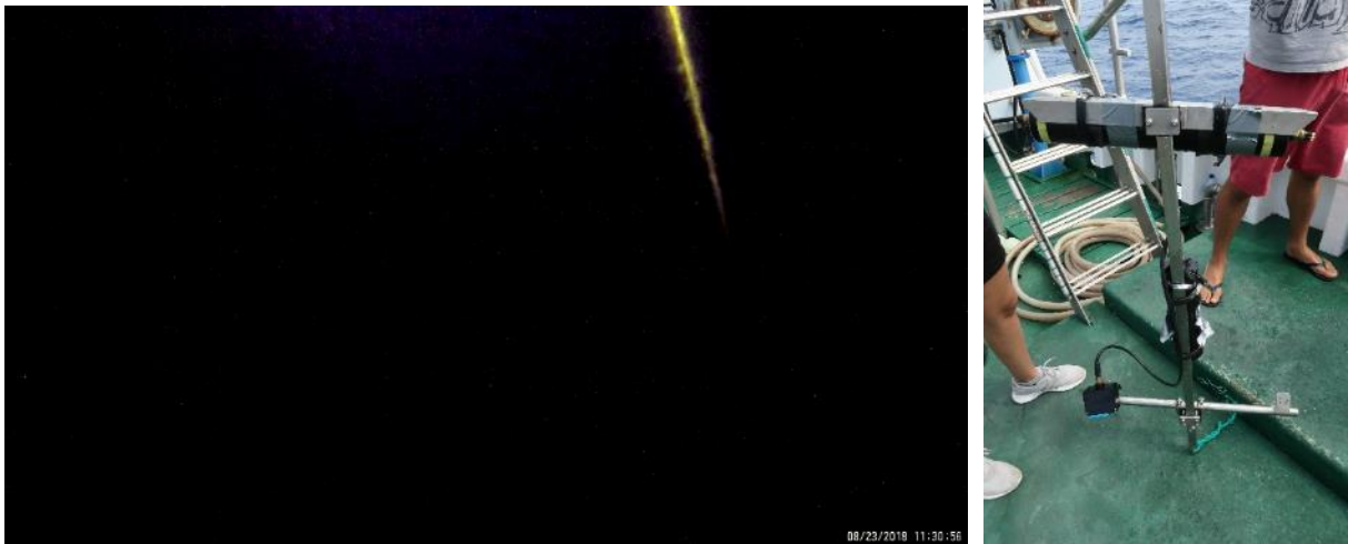
Fig. 15. Long line where the drop-down system got entangled (left) and state of the system after being recovered from the fishing line, with one camera housing and two lights missing (right).
