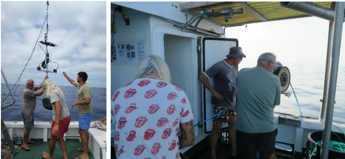
Fig. 3. The vessel's crew deploying the drop-down camera system (left) and controlling its depth using a hydraulic winch. The configuration of the system on the vessel proved successful from day 1.
