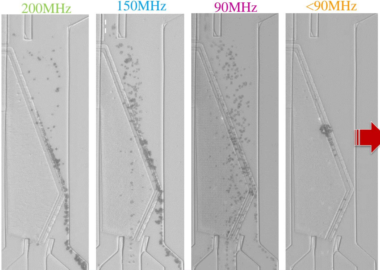
*Improvement to limit cell clogging are still required: Electrodes surface treatment*
