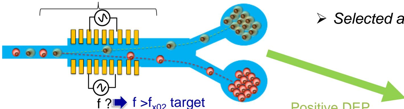
➤ Selected approach: gradual cell deviation using single frequency biasing
