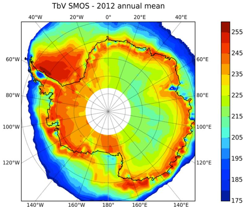
Figure 2-1: Annual SMOS  $T_B$  (K) at V-polarization for  $55^\circ$  of incidence angle in Antarctica.
