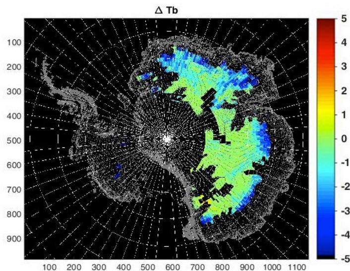
Figure 3-5: Difference between simulated  $T_B$  and SMOS over Antarctica. Values are obtained averaging the  $T_B$  over the incidence angles used for the retrieval.
