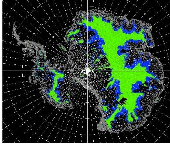
Figure 3-3: Mask of applicability of the ice sheet temperature profile retrieval. The green and blue areas indicate surface balance mass velocity lower than 5m/yr and between 5 and 10 m/yr respectively, standard deviation of  $T_bV$  lower than 1K, ice thickness higher than 1000 m.
