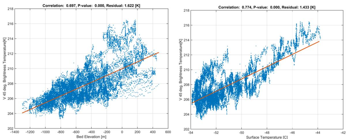
Figure 3-18:  $T_{BV}$  versus bed elevation (left) and  $T_{BV}$  versus -10 m temperature (right).
