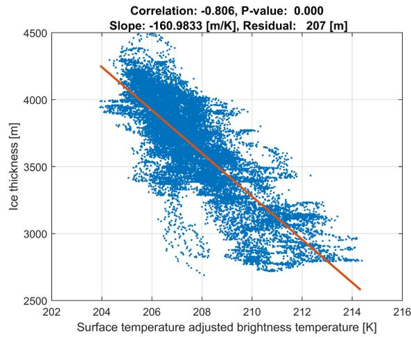
Figure 3-20: Ice thickness vs. SMOS  $T_B$  adjusted for surface temperature in the test area.
