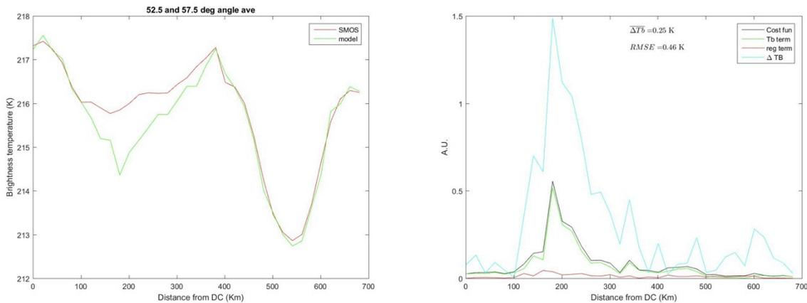
Figure 3-4: (left) Measured (red) and fitted (green)  $T_B$ V, and (right) the Cost Function (black) and its components  $Tb\_MSE$  (green) and regularization term (red), along the transect from Dome C to Vostok Lake. The difference between measured and fitted  $T_B$ V (light blue) is also superimposed to the Cost Function.
