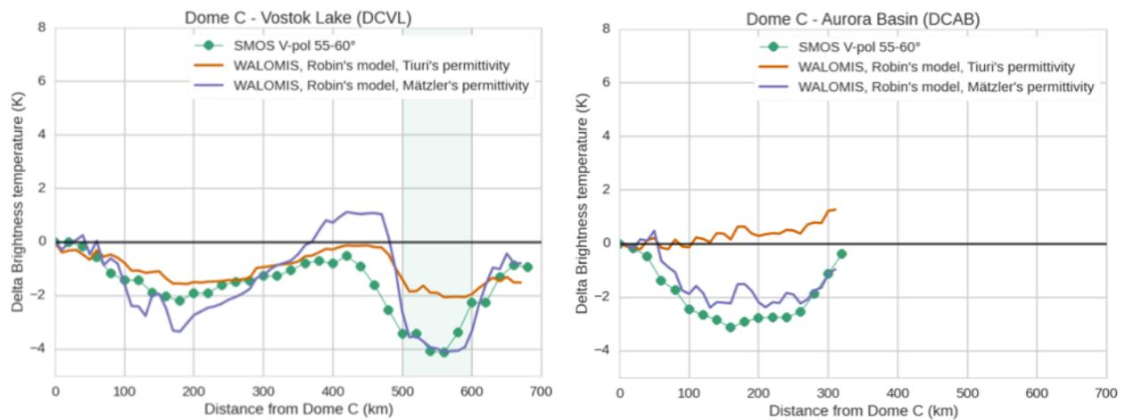
Figure 3-1:  $\Delta T_B$  (i.e.  $T_B$  along the transect -  $T_B$  measured at Dome C) at V polarization for SMOS (green dotted line), and WALOMIS simulated  $T_B$  (orange = Tiuri's permittivity; purple = Mätzler's permittivity) as a function of the distance from Dome C along two transects. The shaded blue area indicates Lake Vostok (from Macelloni et al. 2016).
