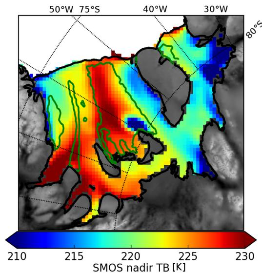
Figure 3-24: SMOS near nadir  $T_B$  ( $<40^\circ$ ) from 2010 to 2015 at the Ronne-Filchner Ice Shelf region with contour of significant amounts of marine ice (Lambrecht et al., 2007). In addition the grounding and coast lines (black) from the MODIS Mosaic of Antarctica project 2009 and the land topography from Bedmap2 (shades).
