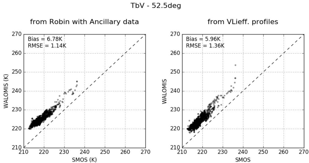
Figure 3-9: Differences between SMOS and the WALOMIS T<sub>b</sub> simulated with temperature profile (left) from Robin model and a-priori data, (right) from glaciological model.
