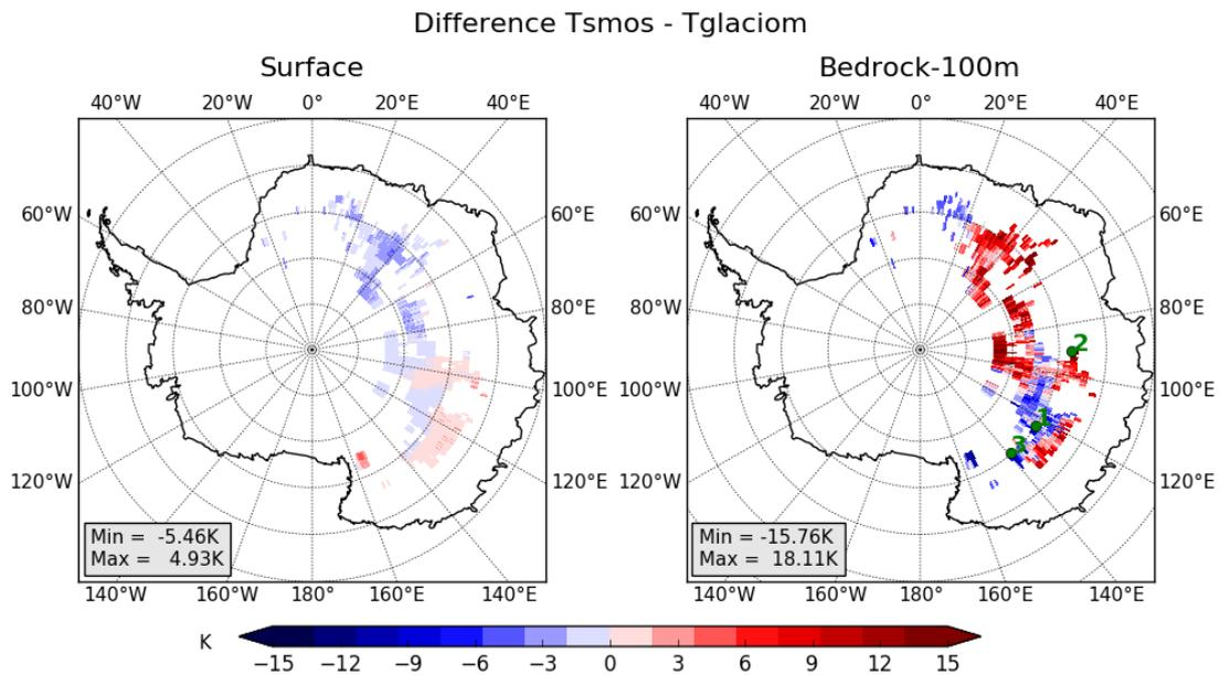
Figure 3-11: Differences between the ice sheet temperature computed from SMOS and derived from glaciological model at the surface (left) and at 100 m far from the bedrock (right).
