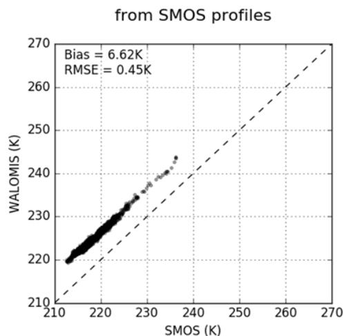
Figure 3-10: Differences between SMOS and the WALOMIS T<sub>b</sub> simulated the temperature profiles obtained after the minimization.
