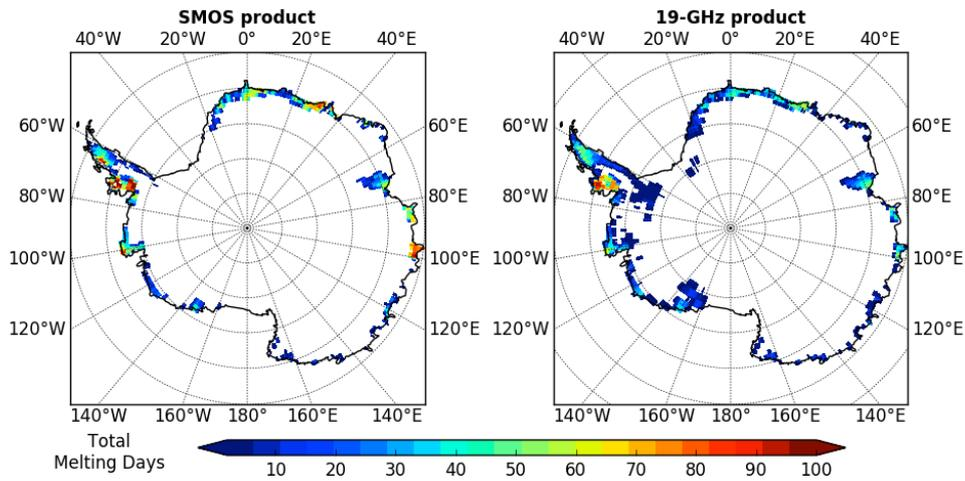
Figure 3-34: Maps of duration of melting period detected by SMOS (right) and 19 GHz (left) melting products for the 2012-2013 season.
