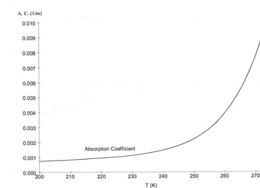
Figure 3-16: Absorption coefficient per meter in ice.
