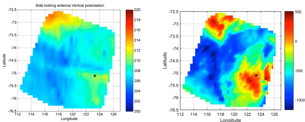
Figure 3-14:  $T_BV$  (K) map of the Concordia are (left) and bedrock in m above sea level (right).
