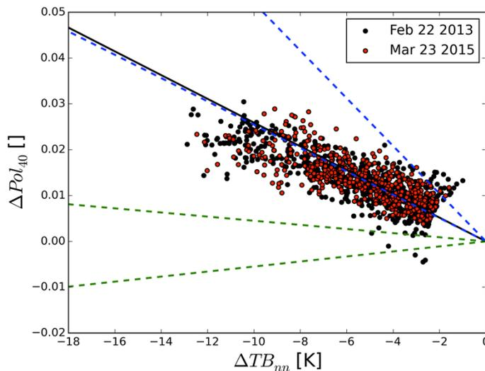
Figure 3-31: Changes in SMOS intensity and polarization by the two surface events highlighted in Figure 3-30 with mean direction of all observations (black line). For comparison, range of model predictions of surface (blue) and bottom (green) intensity to polarization ratios (dashed lines).
