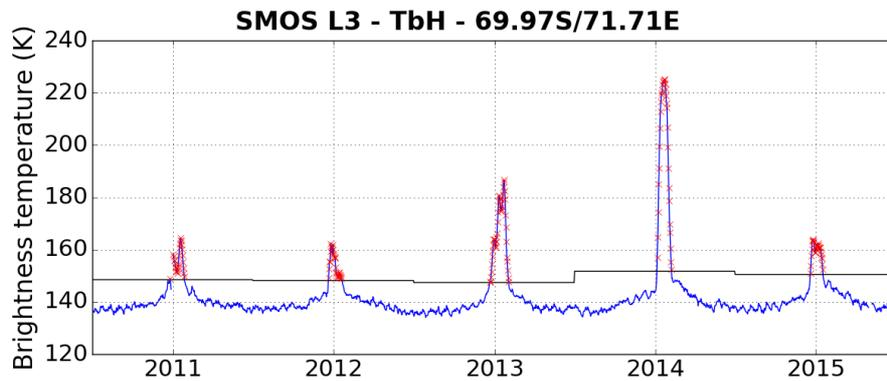
Figure 3-33:  $T_B$  at H polarization (K, blue) from SMOS at 69.97°S, 71.71°E from July 2010 to June 2015. Threshold defined by the algorithm is represented in black and the detected melting days are in red stars.
