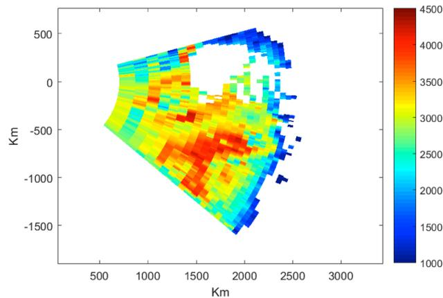
Figure 3-21: East Antarctica area Bedmap ice thickness (m).
