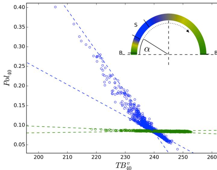
Figure 3-25 Model results (points) varying only near surface parameters (blue) or bottom parameters (green) with 2.5 and 97.5% quantiles of repeated orthogonal regressions on six randomly chosen points (dashed lines). The inlet illustrates the definition of a color scale based on the quantiles.
