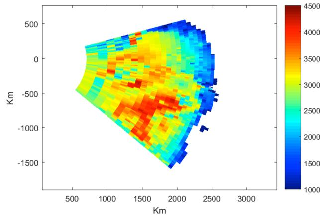
Figure 3-23: Bedmap ice thickness patched using SMOS data.
