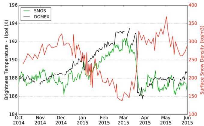
Figure 3-32:  $T_{bH}$  with SMOS at  $52.5^\circ$  incidence angle (green) and DOMEX at  $42^\circ$  (black), and surface snow density in situ measurements (red) at Dome C, Antarctica from October 2014 to May 2015.
