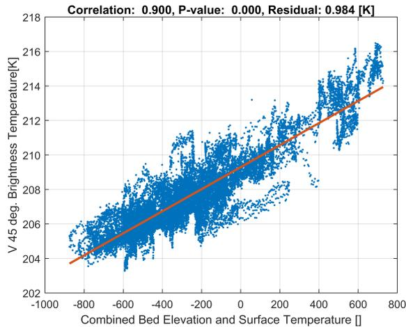
Figure 3-19:  $T_B V$  versus combined bed elevation and surface temperature.
