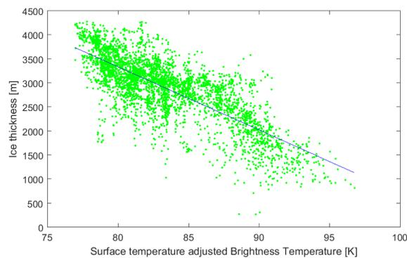
Figure 3-22: East Antarctica area ice thickness vs. SMOS  $T_B$  adjusted for surface temperature.
