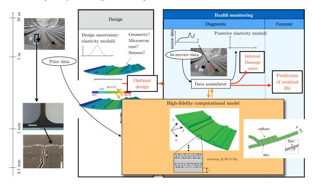
Figure 2.1: The digital twinning concept. A computer model of a physical engineering systems accompanies its physical couterpart and mimics its behaviour. At any time, the virtual twin may be interrogated to predict unobservable quantities, such as the development of hidden defects or the prediction of the evolution of identified defects in the future.
