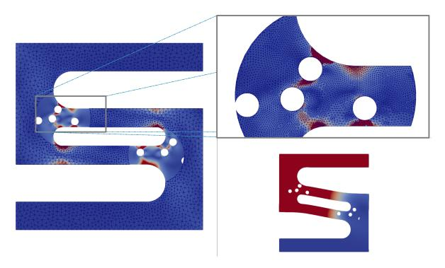
Figure 5.4: The "Zoom" FEM multi-resolution methodology. A fine regular finite element mesh is easily obtained by hierarchical refinement of a coarse grid. One may adapt the level of local resolution by simply evolving the (coarse) level-set that desribes the interface between micro and macro regions.
