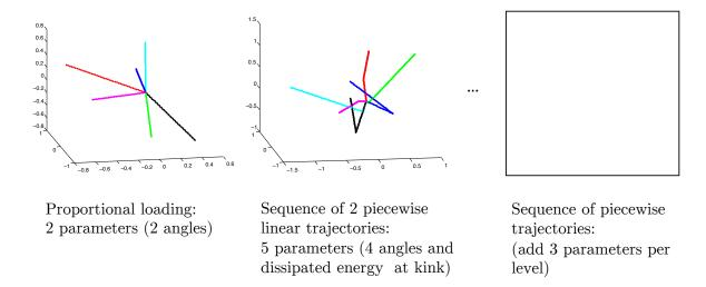
Figure 3.4: Hierarchical snapshot generation for the computational material point problem (from [17]). Optimisation is performed in spaces of increasing dimensions so as to maximally decrease the error of ROM projection.
