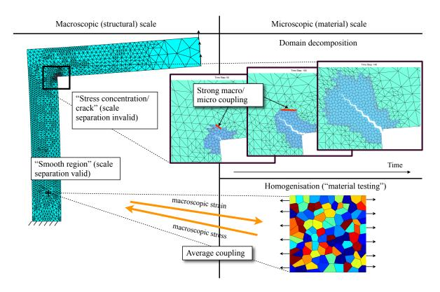
Figure 2.2: Adaptive multiscale fracture modelling, from [8]. Nonlinear computational homogenisation (FE<sup>2</sup>) is used away from the crack. Explicit microscale modelling is used in the damaged regions. The model adaptation is driven by an estimate of the modelling error due to the homogenisation process.
