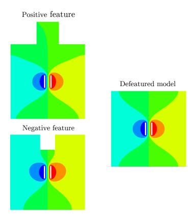
Figure 4.4: Defeaturing approach. We are to estimate whether ignoring negative or positive geometrical features impacts the quality of the output of the numerical analysis or not, without computing the fully featured solution.
