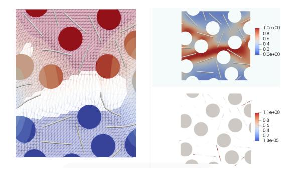
Figure 5.3: Unidirectional elastic fiber elements embedded in a damageable matrix. The bond between the fibers and the matrix is inelastic, and yields above a certain level of axial force. A dedictated LaTIn algorithm is deployed to solve the coupled problem in primal/dual form.
