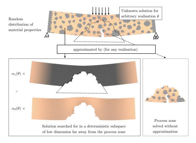
Figure 3.2: Restricted projection-based Reduced Order Model (from [15]). Subspace projection is only performed away from cracks. The damaged regions are found algebraically, using a measure of correlation between snapshot vectors, together with a dedicated greedy methodology, to progressively "eat-way" zones that should not be reduced.
