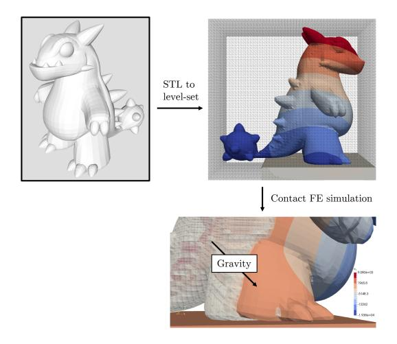
Figure 5.2: Digitial pipeline from geometrical data to FE analysis. The 3D STL Model was created by ThinkerThing to be 3D printed. Only the surface mesh of the component is avaliable. The quality of this mesh is insufficient for analysis purposes. An analysis-ready geometrical description is recovered through the construction of a finite element level-set, which constitutes the starting point of a "Cut" FE analysis.
