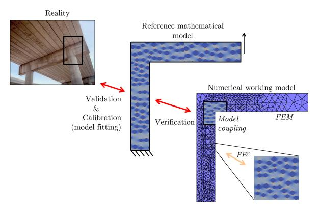
Figure 4.1: Verification and validation of numerical models.
