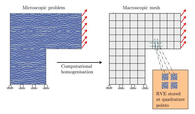
Figure 3.3: The FE<sup>2</sup> approach. High-fidelity numerical material point models are used in stead of macroscopic material laws. The time evolution of these material point problems needs to be calculated at every quadrature point of macroscopic meshes, leading to tremendous computational cost. Fortunately, material point problems can be algebraically reduced.
