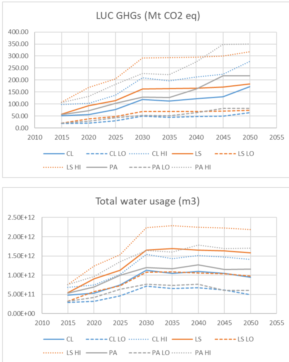
Figure 37. Projected biomass production [PJ] by pathway and the associated land use change emissions and water usage. In the case of biomass-induced GHG emissions due to land use change, full lines indicate a median estimate whereas (LO, HI) indicates estimates calculated using conversion factors corresponding to the 25 th and 75 th percentiles, i.e., providing an estimate of the uncertainty. For total water usage the corresponding values correspond to the mean estimate and (-/+ ) one standard deviation.
