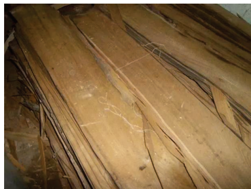
Fig. 6. Raw dried oak veneer with humidity W=6 % and weight m_d=4.41 kg
